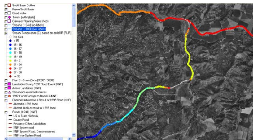
Figure 33. This map shows summary data of Scott River Thermal Infrared Radar (TIR) surveys for Shackelford Creek. Note that water temperature warms in a downstream direction as flow is depleted. Reaches with no temperature coded color are dry, indicating loss of surface flow in violation of CDFG Code 5937 and over-diversion in violation of SWRCB Codes 1243, and 1375. Data from Watershed Sciences (2003).
